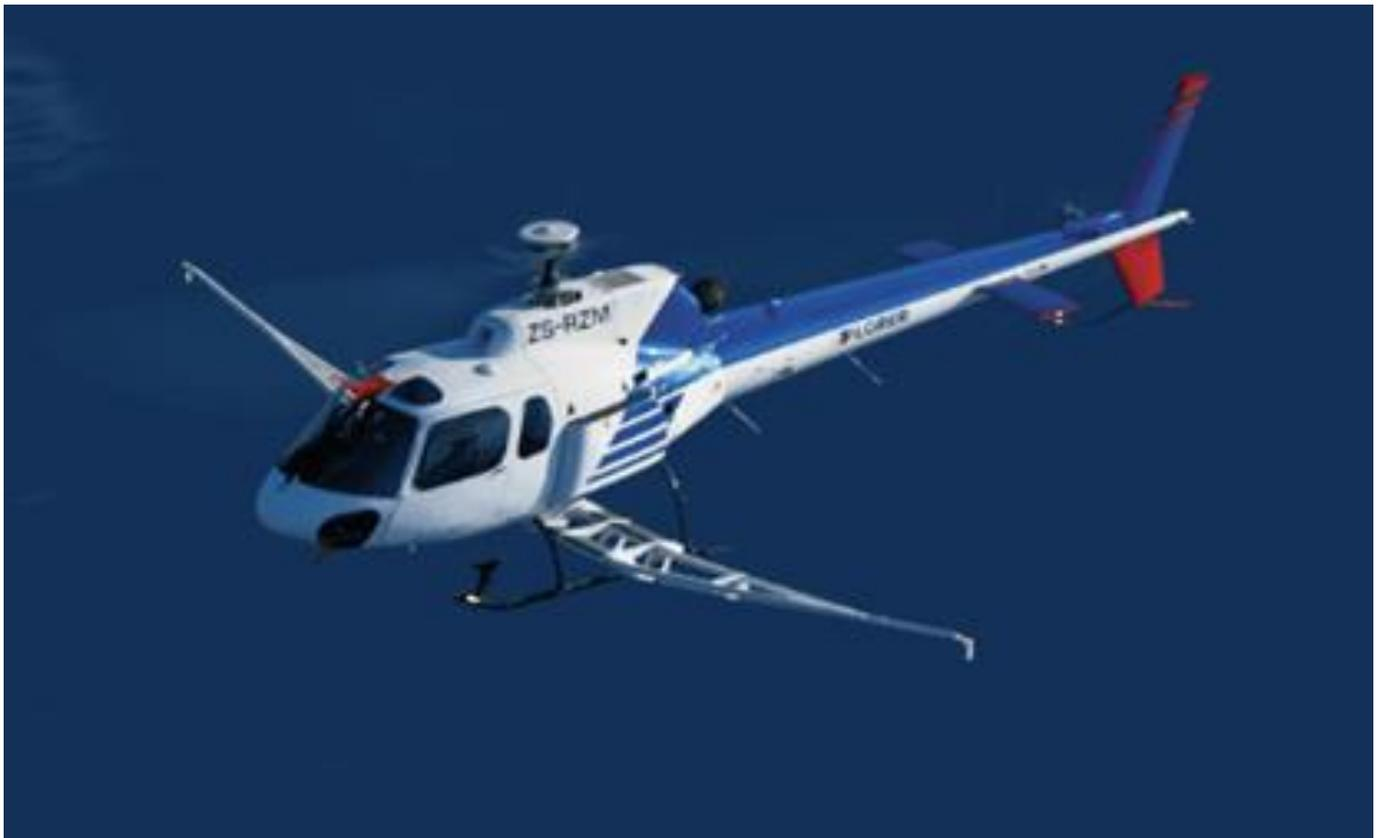
**Figure 6.** NRG's Xplorer™ heli-borne gradient magnetometer system proposed to complete a detailed magnetic survey over the Dittmer project area and funded by a Queensland State Government CEI grant.
