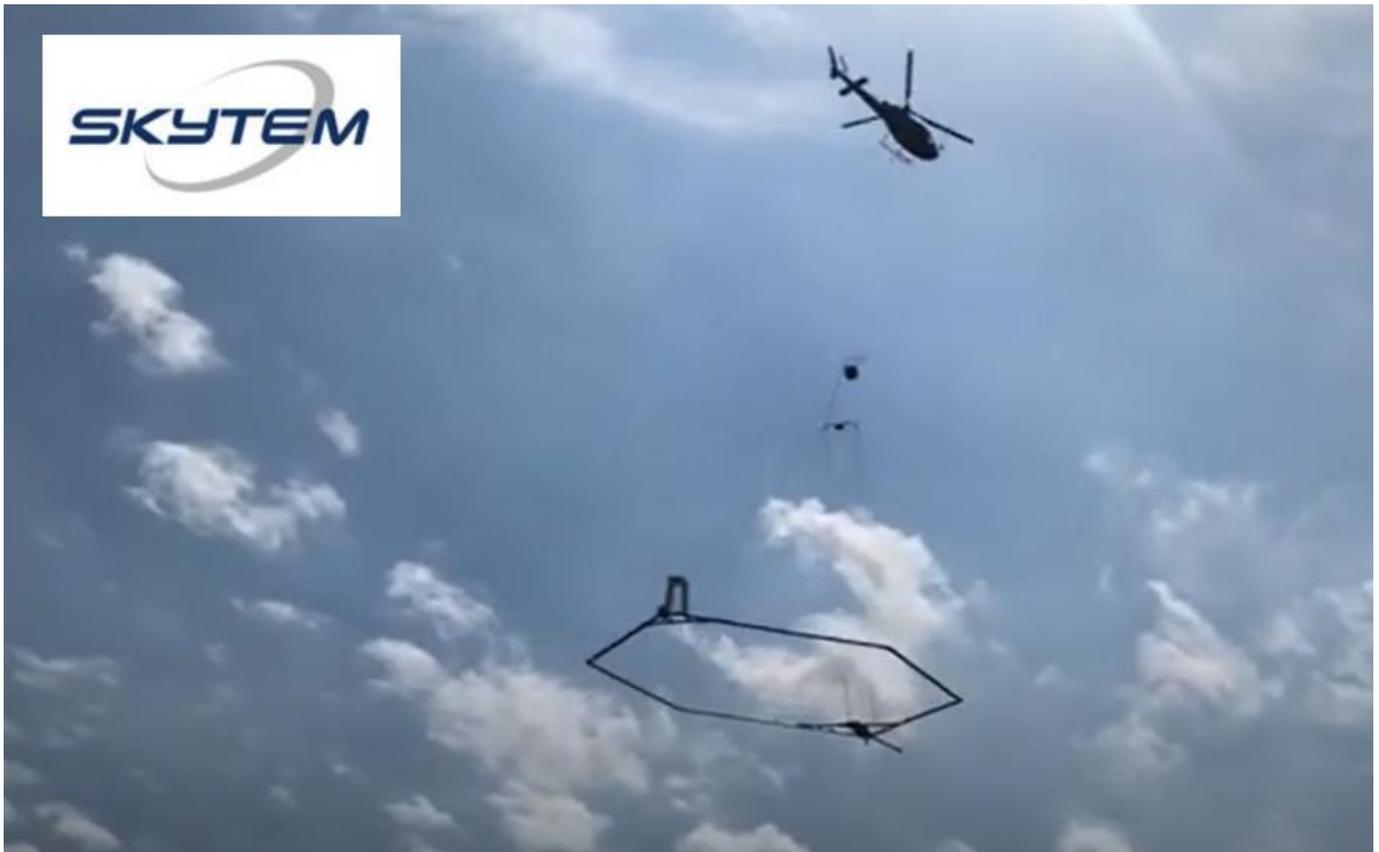
**Figure 7.** SkyTEM's low-frequency time domain EM and magnetic system. proposed to complete a detailed heli-borne EM survey over the Maniopota prospect (Ruddygore Project) and funded by a Queensland State Government CEI grant.
