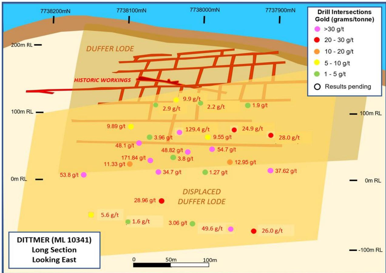
**Figure 3** – Long section looking east at the Dittmer Mine area showing significant gold drill intersections to date.
