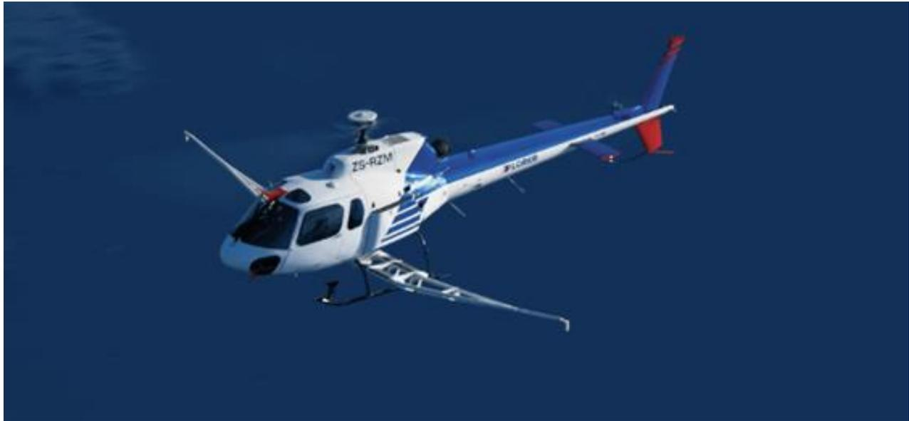
**Figure 1-** Example of an ASTAR B-series helicopter using the Xplorer™ heli-borne gradient magnetometer system proposed to complete the survey.
