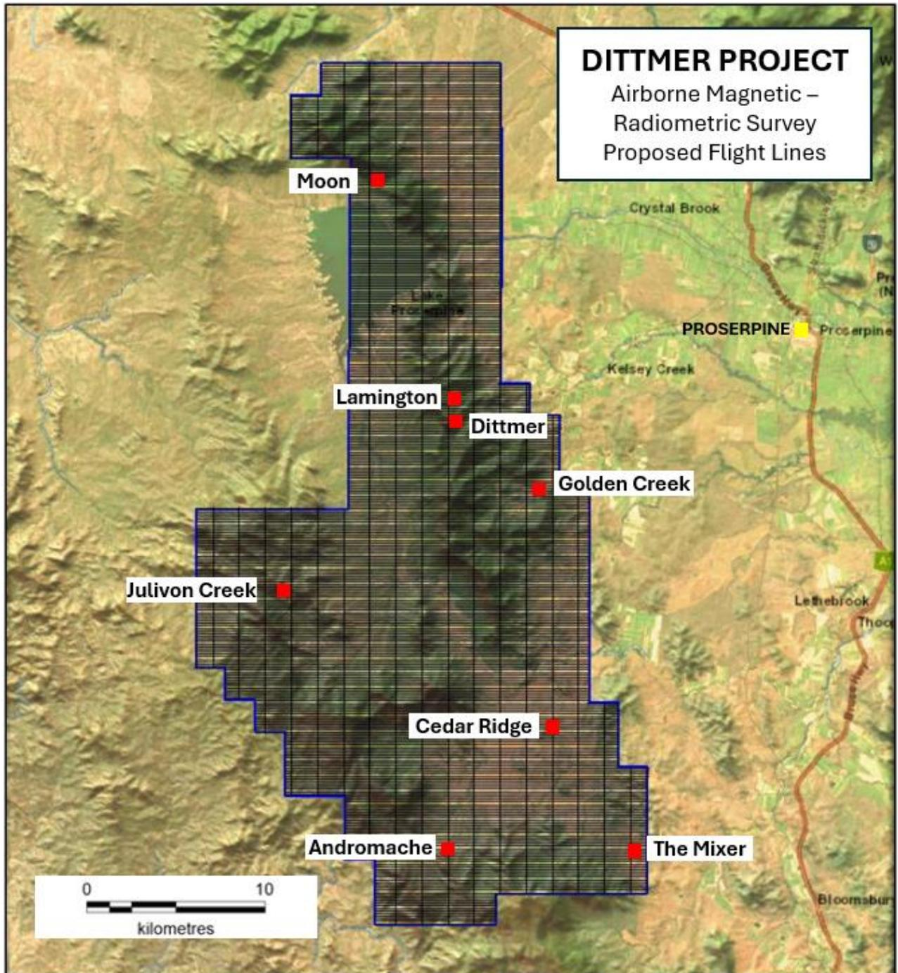
*Figure 3 - Proposed Dittmer Project airborne survey flight lines.*
