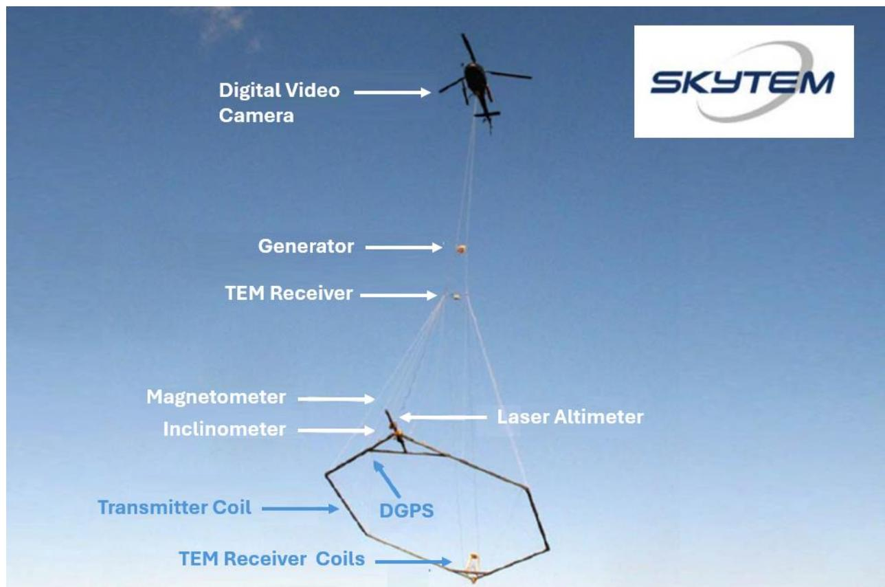
**Figure 4** - Example of the heli-borne EM system configuration for SkyTEM’s Low-frequency Time Domain Electromagnetic and Magnetic system.
