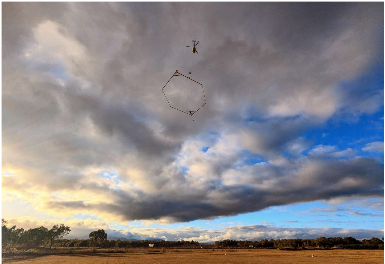
Figure 6 – SkyTEM heliborne EM survey being undertaken at Mount Molloy
