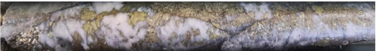
Drill core from drill hold DTDD009 showing quartz-chalcopyrite vein material grading 171.8g/t Au, 56.4 g/t Ag and 5.28% Cu (See ASX Announcement 4 July, 2023).
