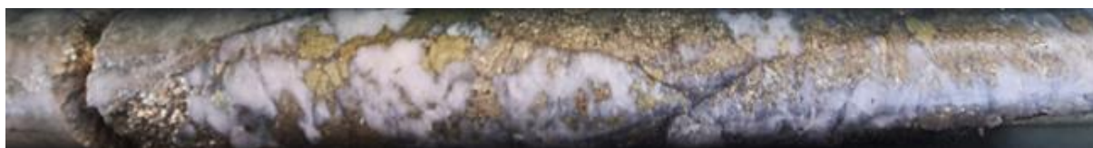
Figure 4: Drill core from drill Hole DTDD009 showing quartz-chalcopyrite vein material grading 171.8 g/t Au, 56.4 g/t Ag & 5.28% Cu
