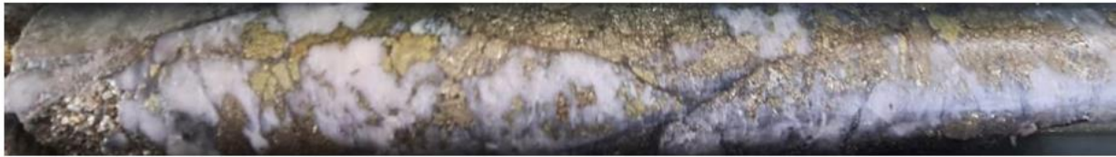
Figure 2 – Drill core from drill hole DTDD009 showing quartz-chalcopyrite vein material grading 171.8g/t Au, 56.4 g/t Ag and 5.28% Cu
