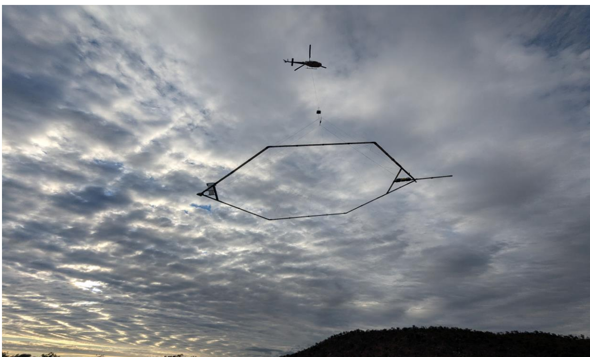
Figure 9. SkyTEM's EM and magnetic system. Surveying the Mount Molloy area.
