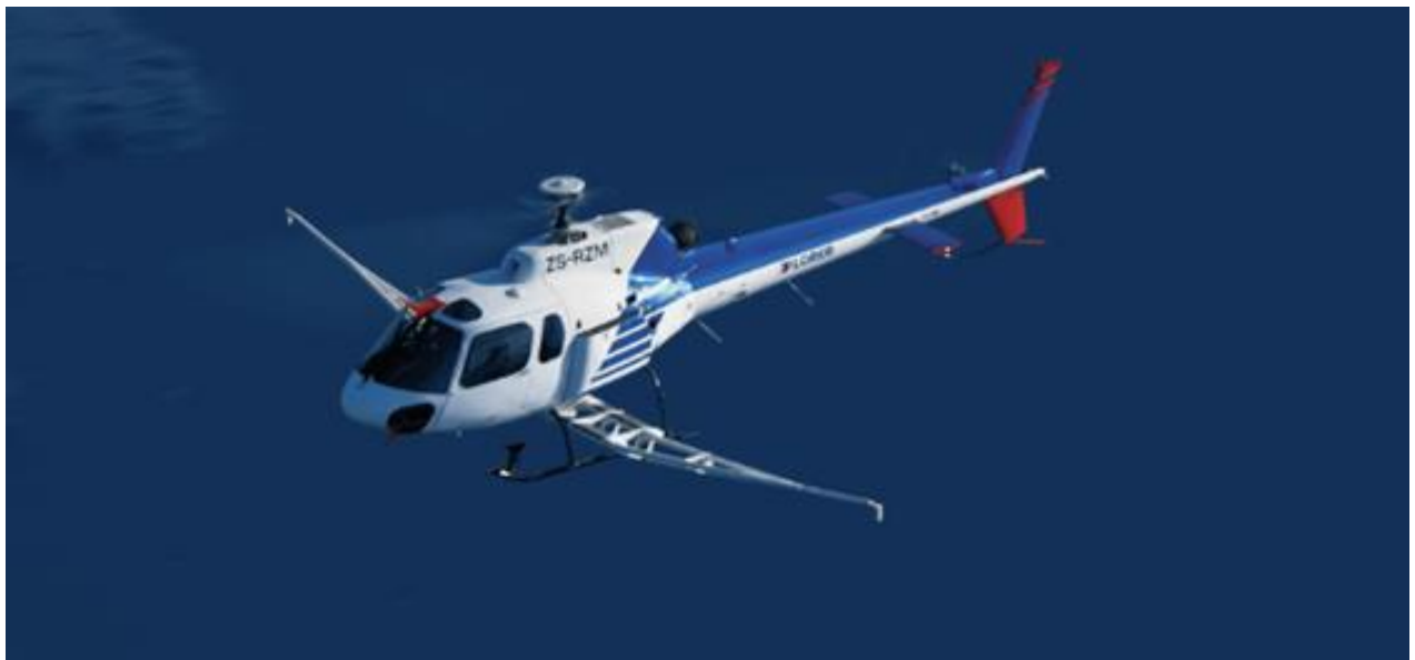
Figure 5- Example of an ASTAR B-series helicopter using the Xplorer™ heli-borne gradient magnetometer system proposed to complete the survey.
