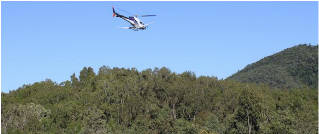
Figure 2 – NRG’s Xplorer™ heli-borne magnetic survey being flown over the Dittmer project area and funded by a Queensland State Government CEI grant.
