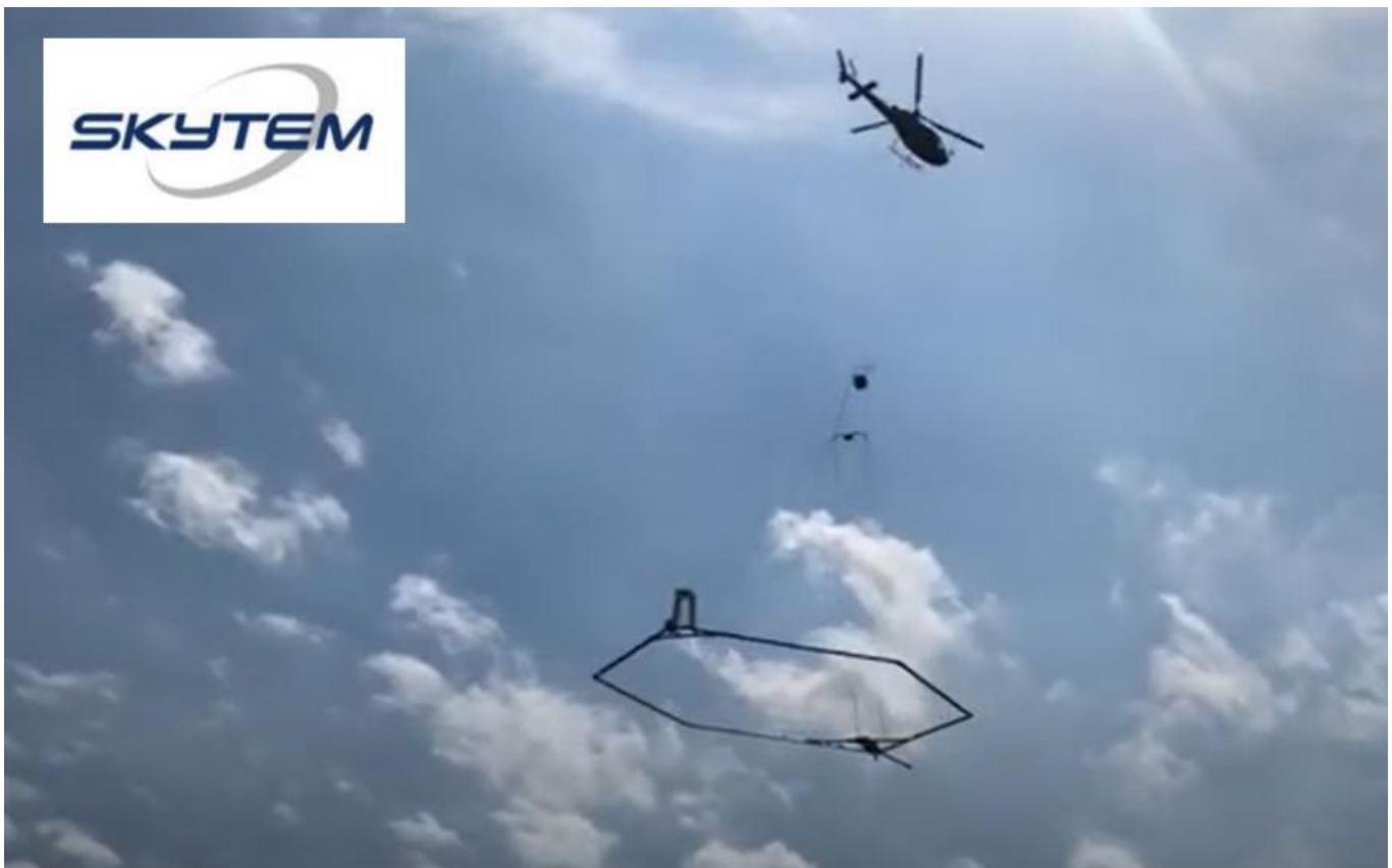
Figure 9 - SkyTEM's low-frequency time domain EM and magnetic system. proposed to complete a detailed heli-borne EM survey over the Maniopota prospect (Ruddygore Project) and funded by a Queensland State Government CEI grant.
