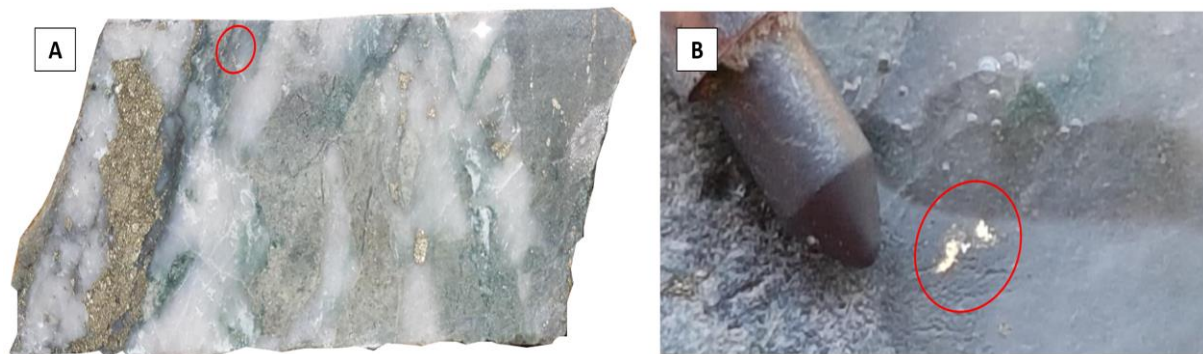
Figure 2. (A) Quartz-pyrite-chlorite vein in DTDD007 (97.8 – 98.0m) with visible gold circled; (B) Close-up of visible gold
