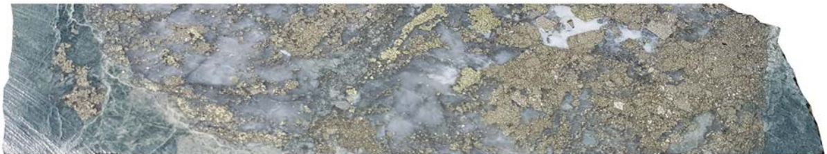
Figure 4. High grade drill intersection of quartz-carbonate-pyrite-chalcopyrite in DTDD004 (215.4 – 215.9m) that reported 0.5m @ 9.57 g/t Au, 16.8 g/t Ag and 0.68% Cu.
