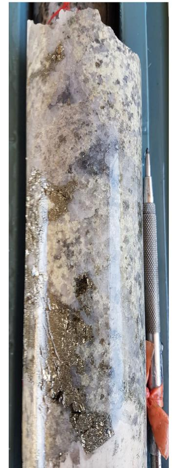
*Drill hole BSMDD001 completed at 351.04m and intersected broad zone of milled and crackle breccia*
