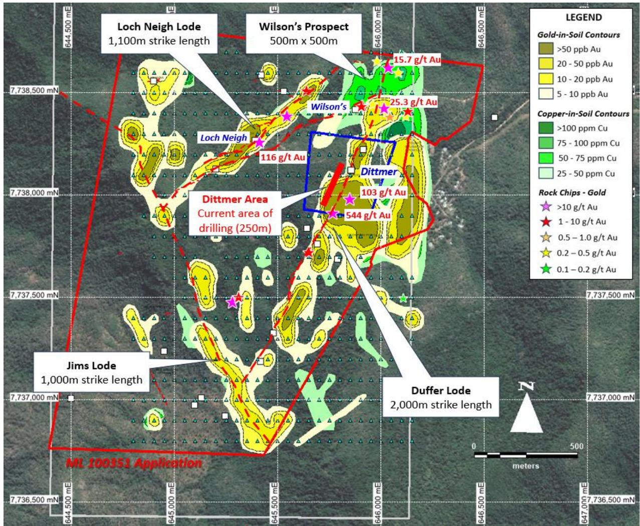
**Figure 1** – Plan view of the Dittmer prospect area with gold and copper-in-soil anomalies and significant rock chip results.
