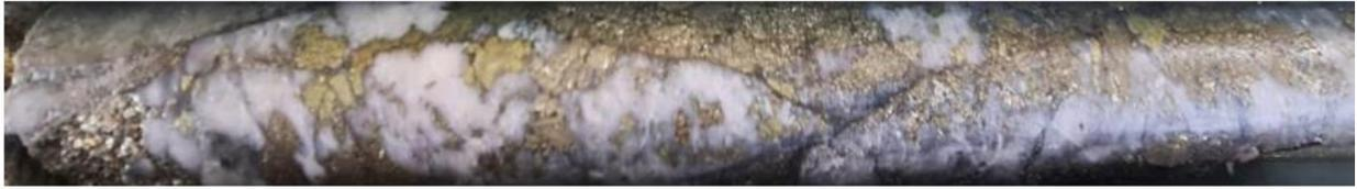
**Figure 6** – Drill core from drill hold DTDD009 showing quartz-chalcopyrite vein material grading 171.8g/t Au, 56.4 g/t Ag and 5.28% Cu
