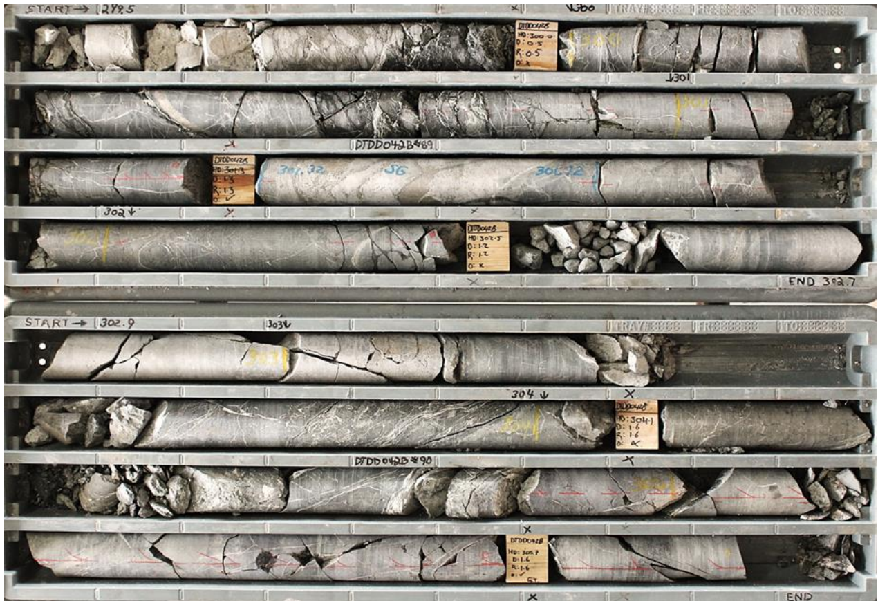
Figure 1 – Ore zone in DTDD042B (299.5 – 304.3m) including quartz-carbonate-chalcopyrite-pyrite veins within sheared, silicified volcanics 2 .
