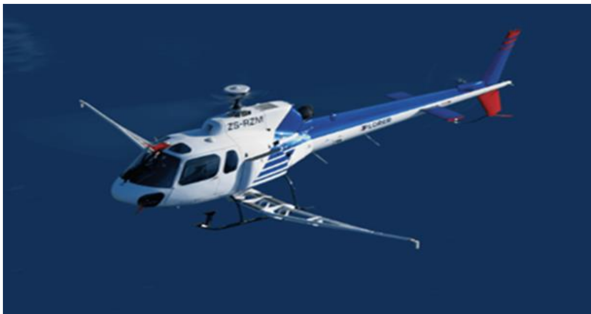
Figure 4 – Example of the Xplorer™ heli-borne gradient magnetometer system scheduled to survey Dittmer.
