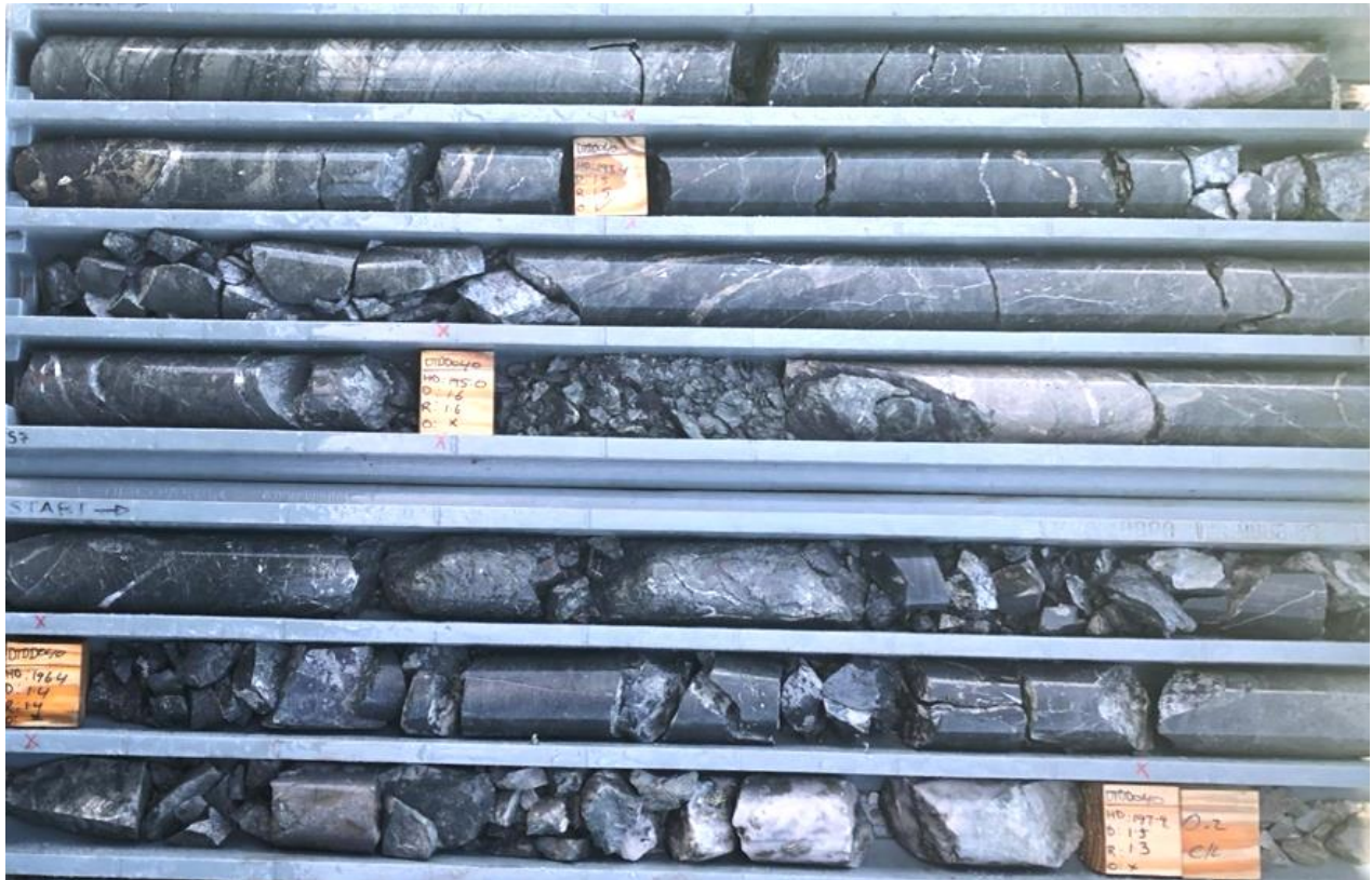
Figure 1 – Ore zone in DTDD040 (193 – 201m) including quartz-carbonate-chalcopyrite-pyrite veins within sheared, silicified volcanics.
