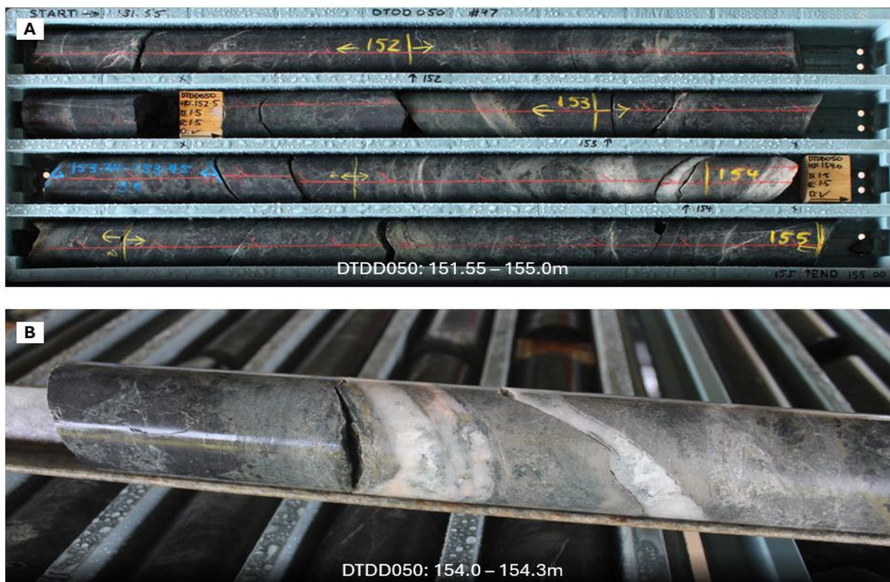
Figure 4 – Examples of mineralisation in DTDD050; (A) Core tray exhibiting the greater Displaced Lode structure; (B) Close-up of the quartz-pyrite-chalcopyrite veins up to 40mm in phyllic altered andesite.
