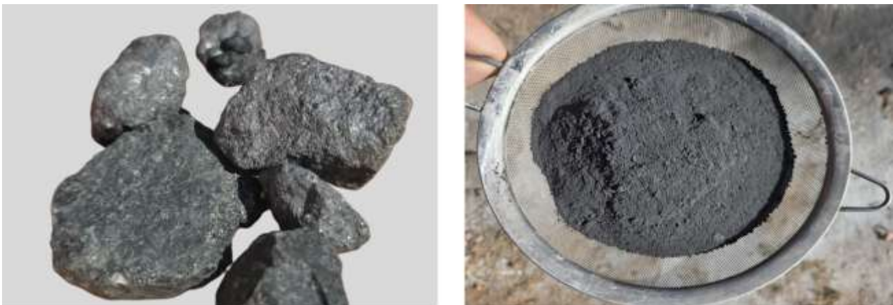
Figure 2 – Galena and sphalerite mineralisation percussion chips intersected in BTPRC010 (90 – 91m)
