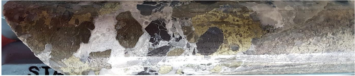
Figure 2. Close-up of quartz-carbonate-pyrite-chalcopyrite-sphalerite vein (BRUDD001: 13.9 – 14.1m)
